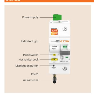
EKR3S Smart MCB offers overload and short-circuit protection for circuits up to 100A, and can also monitor various electrical parameters in real-time, with remote control capabilities through the Tuya APP or RS485 platform.
