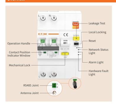
EKRO Smart RCBO combines the functions of traditional circuit breakers with modern electronic technology to provide overload, short circuit, and leakage protection for circuits rated at 63A. It also supports remote control through the Tuya App or RS485 communication platform, allowing monitoring and adjustment of various electrical parameters. The EKRO Smart RCBO has been widely used in smart building power management, industrial power monitoring, and energy efficiency optimization.
